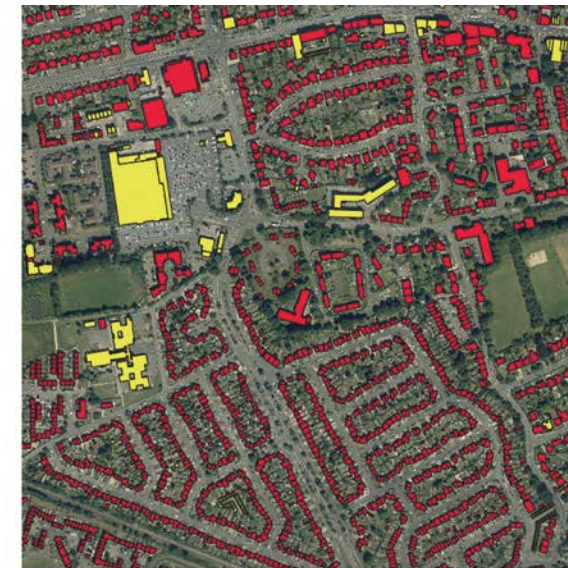
Left: Results from the roof face estimation algorithm. The individual roof faces are shown shaded by their aspect (e.g. yellow is North, dark purple is East). The outline of each building is coloured by how accurate the algorithms results are - these are summarised for the whole test region in the histogram underneath. Right: Results of the flat vs pitch (not-flat) algorithm for a district of Newcastle.
