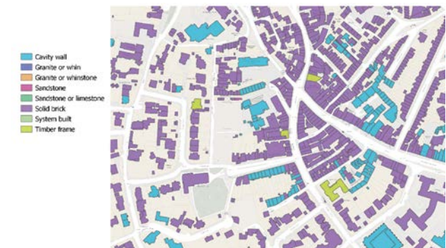
Wall Construction Results in Camden Test Region
