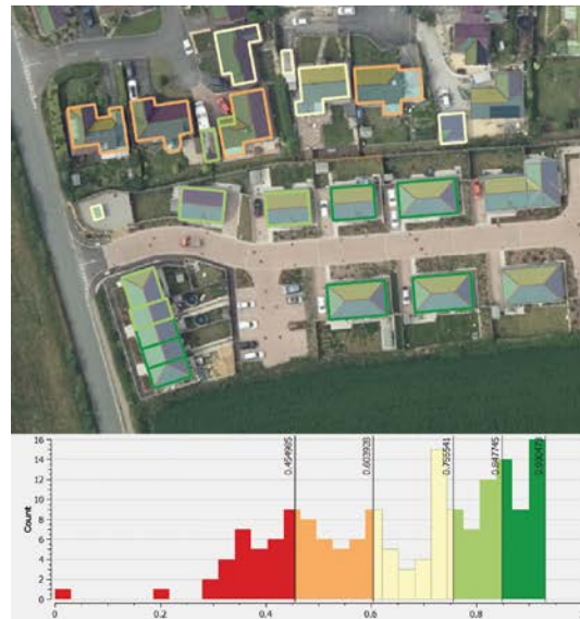
Left: Results from the roof face estimation algorithm. The individual roof faces are shown shaded by their aspect (e.g. yellow is North, dark purple is East). The outline of each building is coloured by how accurate the algorithms results are - these are summarised for the whole test region in the histogram underneath. Right: Results of the flat vs pitch (not-flat) algorithm for a district of Newcastle.
